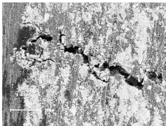
Fig. 5. Cracks and propagation in meat at N = 21216 , \sigma_{\max} = 100 MPa (scale bar is 100 \mu\text{m} ).
